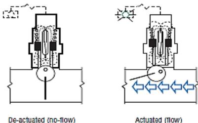
Figure 4 Paddle Type Flow Switch Operation
